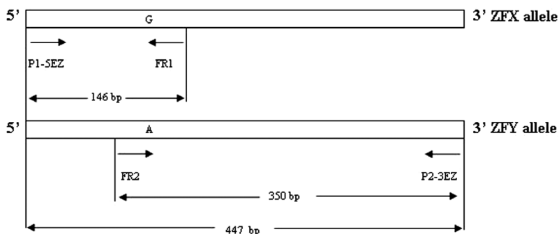
Fig. 1. Principle of the sex determination of giant panda. The polymorphism site used here is a A/G substitution at position 122 of ZFX/ZFY. At the 3' end of the internal confronting primers FR1 and FR2, the base specific to each allele is designed. 146 bp: size of amplicon representing the ZFX allele; 350 bp: size of amplicon representing the ZFY allele; 447 bp: size of amplicons from both ZFX and ZFY.
