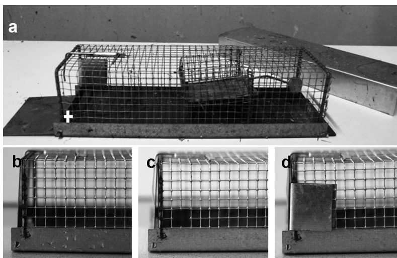
Fig. 1. (a) Open Ugglan special trap No. 2 (Grahn AB; Sweden). White cross indicates location and wires to be removed to provide a shrew exit. (b) Corner of closed trap without a shrew exit, (c) with a shrew exit, and (d) with a shrew-exit clip to close the exit in case the trap is needed for shrew captures (photos: Antje Herde, measures and clips developed by Jana A. Eccard).
